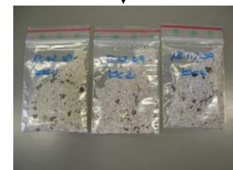
6. Recycling product: CSH after drying
